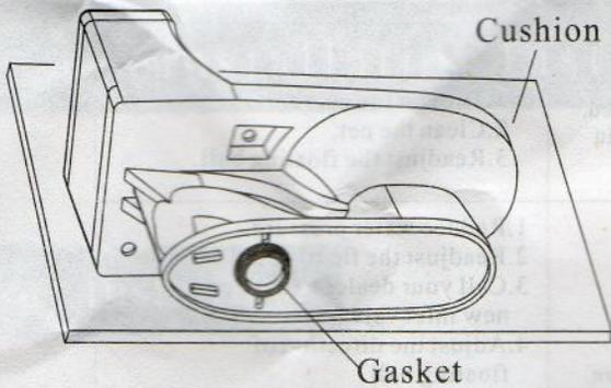
4. Put the product onto the cushion flatly, then place the wax ring gasket onto the drainage outlet tightly.
