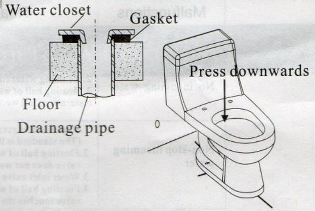
5. Clean the drainage outlet, then put up the toilet to make the its center line aligned with the one on floor and the center of the waste outlet aligned with the center of the drainage outlet. Press the product downwards until it is flat.
