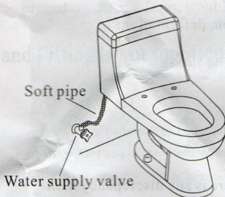
7. Install the water supply valve. Connect the filter and water supply soft pipe of cistern. Check the connection carefully to make sure there is no leakage.
