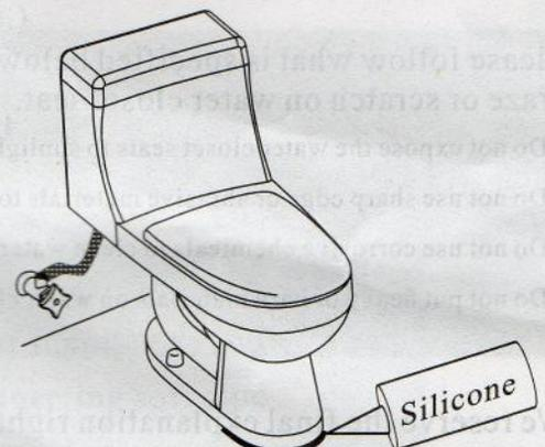
8. Install toilet seats according to the installation instructions, then dab a layer of silicone between the product and floor.
