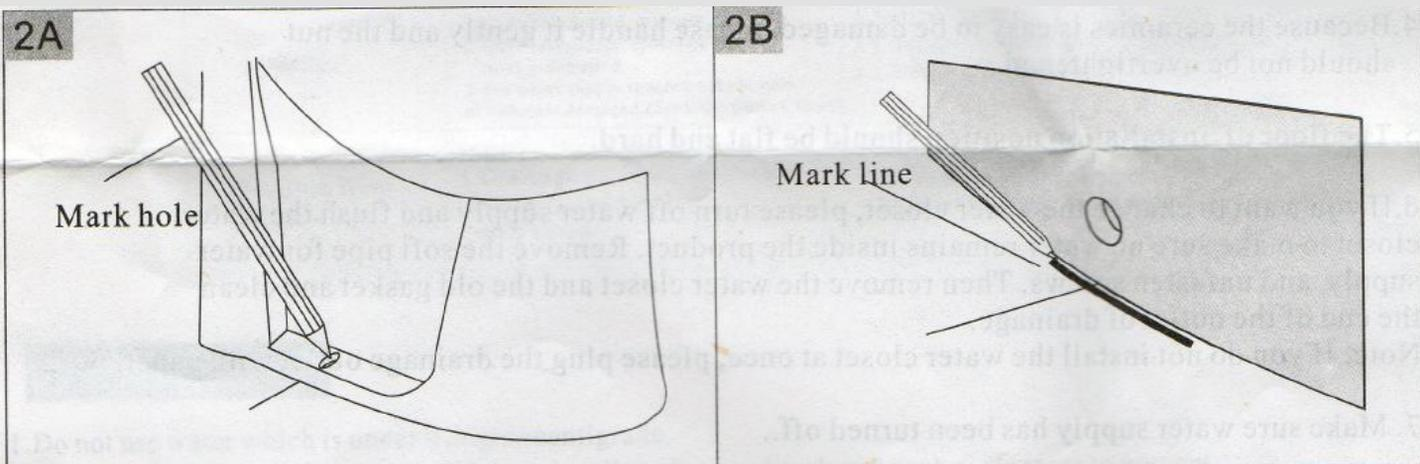
2. Put the toilet into the installation position. Make sure the + center lines of floor and toilet are aligned properly.
