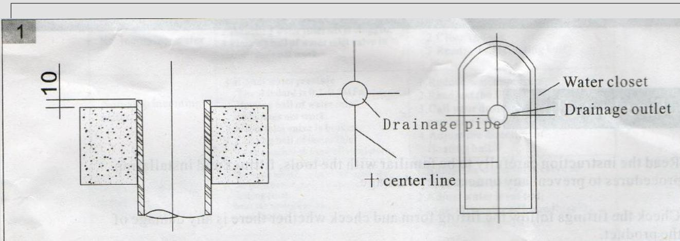
1. Mark the + center line according to the drainage outlet on the floor and that of the toilet.
